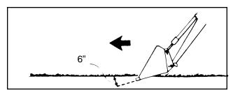
Use a slight bucket angle, travel forward, and hold the lift control forward to start the cut. Make a short, angle cut approximately 6" deep and break-out cleanly.
